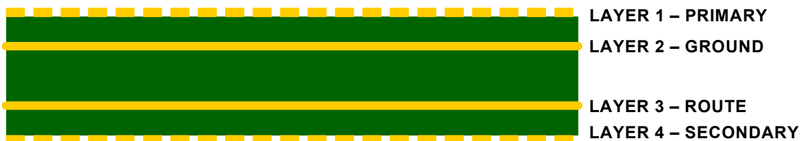
Figure 7. Four Layer Stackup
