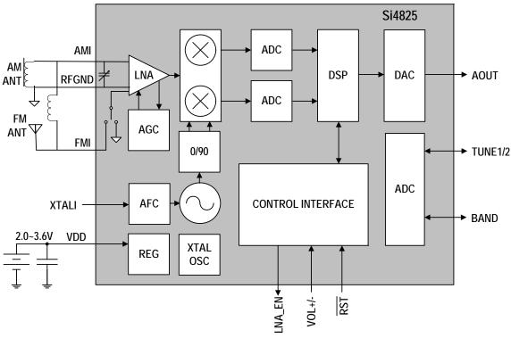
Figure 2. Si4825 Functional Block Diagram
