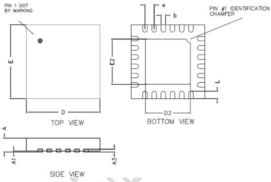
Figure 10 QFN 4x4 24 Pin Package diagram
