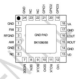
QFN 24 Pin Assignments (Top View)
