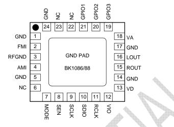
Figure 8 Pin assignment for BK1086/88 QFN24 4x4 mm package
