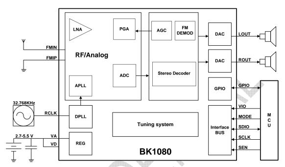
Figure 1 Chip Block Diagram
