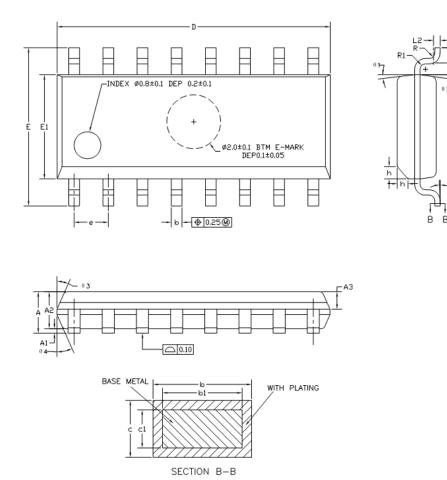
Figure 22 SOP 16 Pin Package diagram
