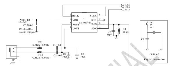
Figure 18. BK1080VB with Single-ended Input Application
