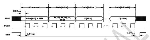
Figure 7 3-wire Interface Diagram
