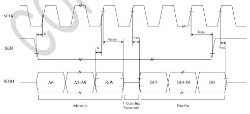
Figure 12 3-Wire Control Interface Read Timing Diagram
