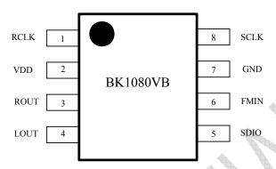
Figure 6 Pin Assignment for BK1080VB package (top view)
