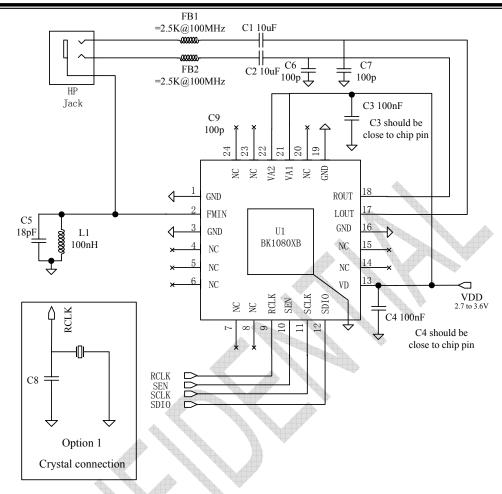
Figure 15. BK1080XB with Single-ended Input Application
