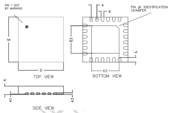
Figure 19 QFN 4x4 24 Pin Package diagram
